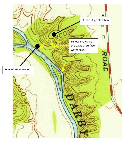
One feature of topographic maps that is not readily evident, but nevertheless provides critical information on surface water flow, is the direction of contour lines in relation to surface water flow. Contour lines are usually smooth, unless the topography shows an abrupt change in elevation or direction. One instance where this abrupt change occurs is when surface water flow is evident.
