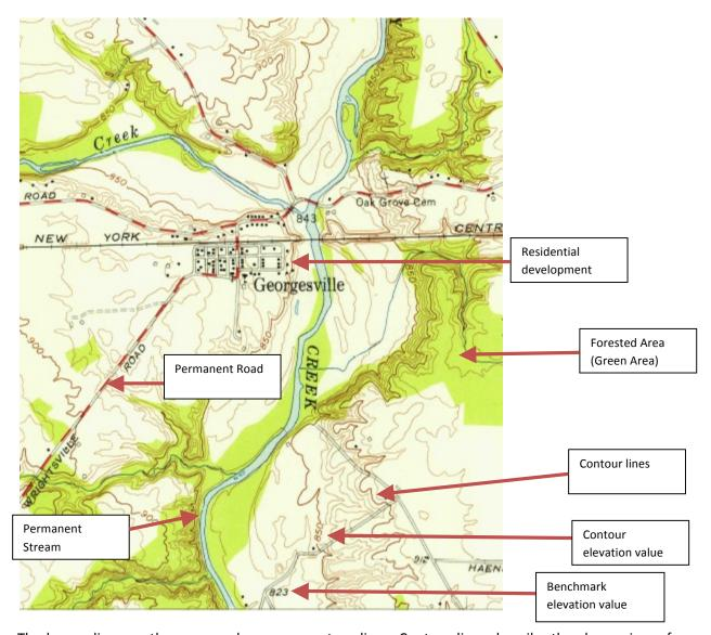
The brown lines on the map are known as <u>contour lines</u>. Contour lines describe the change in surface elevation over a linear horizontal distance. The elevation is indicated by values that are in-line with the contour lines. Elevation is also indicated from benchmarks that are indicated as independent features on the map. Thick contour lines represent significant elevation values, and are usually shown as increments of 50 feet (e.g. 850 feet and 900 feet in this example).
